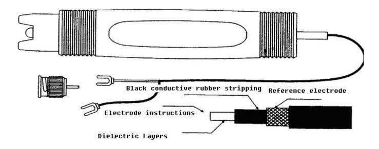
• The electrode's structure picture with temperature
